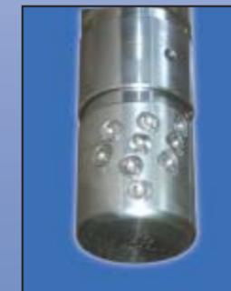
The perforated flow-to-close plug and the nozzle design maintain accurate control of varying process conditions through precise throttling of the cooling liquid control valve in response to feedback from a controller and downstream temperature sensor.
